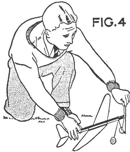
This model will take off the ground without any assistance from the launcher with one row of knots wound up into the rubber motor. No pushing is necessary. Simply place it on the ground and release it. The proper way to hold the model for launching is shown in Fig. 4. Fully wound, it will jump immediately into the air, 275 turns may be put into the motor wound by hand. When stretched and wound with a winder, it may be wound to 550 turns.
