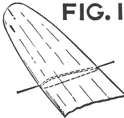
Obtain a piece of sheet balsa measuring at least  $1/32$ " thick,  $2-5/8$ " wide and  $17-3/4$ " long. Study the top view of the wing in the plans under "Wing." This shows the wing as it looks after being bent around its two ribs, as shown under "Wing Section." The width of the wing after bending is  $2-1/2$ ", but the original width must be  $1/16$ " wider to allow for its bend. In this manner, the wing must be cut and its edge sandpapered down to  $2-9/16$ " wide.
