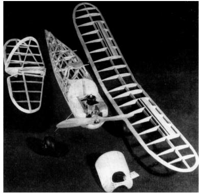
Plane is composed of separate units which are conveniently detachable, facilitating transportation
