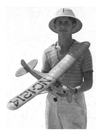
unbelievable. The square fuselage construction allows as much strength as in a cabin type fuselage of the same size, permitting the use of a powerful motor for top performance.
