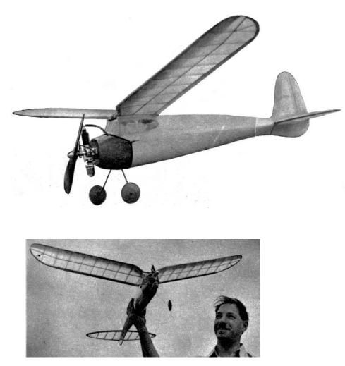
Above -- Garami and the Molecule. Left -- Start of the record flight at Haley Field, where the Molecule outflow larger ships. The monocoque fuselage and wing installation are points to note. Nose detaches.
