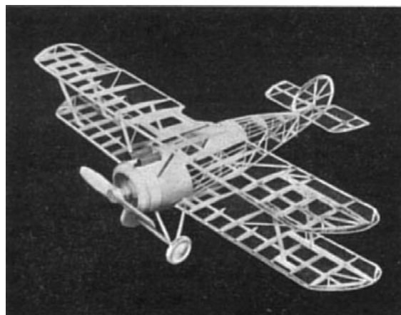
The frame of the Sopwith Camel before covering. This photo will be of service in assembling the model.
