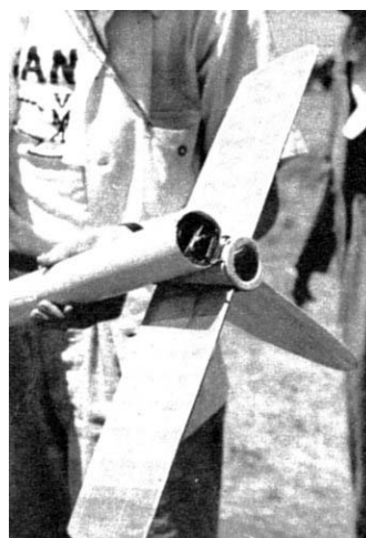
Rear of stick is tinged for easy winding. Rudder is sheet balsa.
