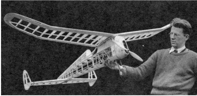
No tricky construction in the Apache. Double rudders are optional. Note wing-tip slots. It's a Class C.
