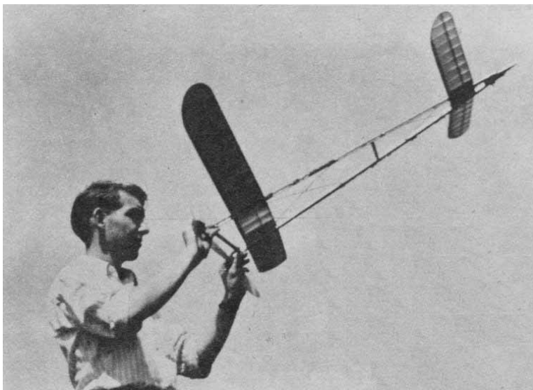
How a twin-pusher is launched. Forte is great longitudinal stability.
