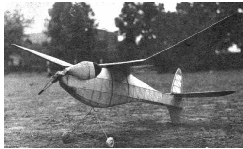
Fuselage is made of primary frame, faired top and bottom with formers.
