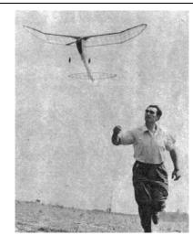
Test glide. Dodger has proper incidences built in, no side thrust, slight downthrust. Climbs wide left circle, glides sharp left circle.
