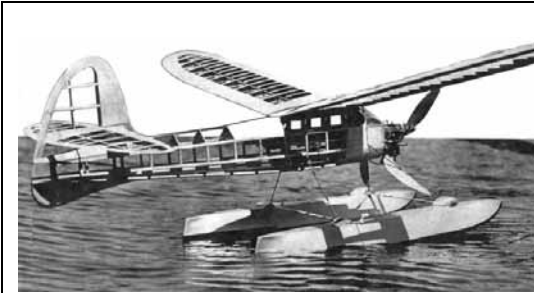
Floats were developed through a series of test models. Wing loading, both models, 11oz.
