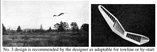
No. 3 design is recommended by the designer as adaptable for towline or hy-start gliders. Slotted aileron was found to greatly increase the model's stability.
