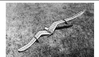
The rubber version of this design produced flights of over a minute and a half. It proved slightly tricky as a gas job; the wings were found too weak.
